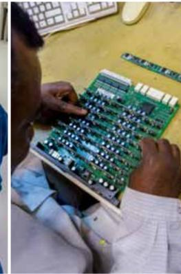
> Repairing boards for telephone exchanges
